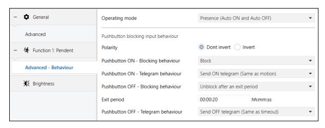
**Approach 2:** The pushbutton is directly linked to the motion sensor and the actuator in one group address. In this setup the pushbutton turns the actuator on directly and just blocks the motion sensor preventing it from timing out.
