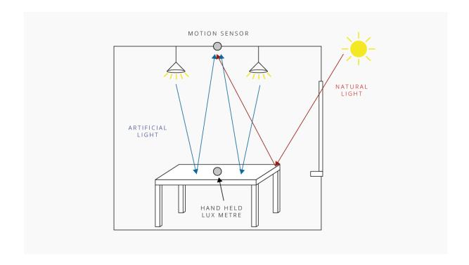
It is therefore necessary to apply a room correction factor to convert lux level received at the sensor to an estimate of the lux level on the desk / floor below the sensor. During factory calibration the sensor is calibrated for an average environment containing desks and carpets, but in reality every environment will be different. Therefore calibration will be necessary to ensure optimal performance.
