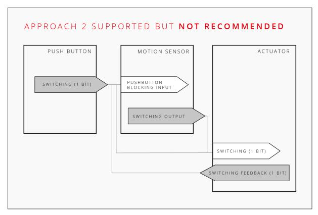
To enable the sensor to be configured in approach 2 the two parameters shown below in red have to be changed to "Do nothing". This will prevent the motion sensor from turning ON/OFF the light directly when receiving a telegram from the push button, it will simply just block the motion sensor.
