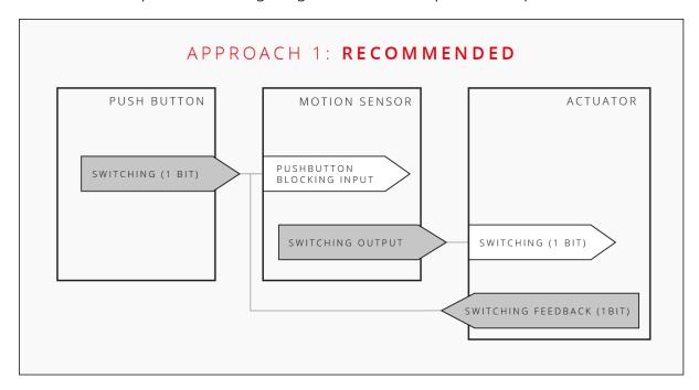
The screenshot below shows the default settings which are designed to work with approach 1, with these settings the sensor is configured to automatically turn the function ON when the sensor detects motion and OFF when the timeout elapses.
